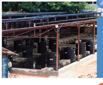
The most critical part of the process, soaking, starts by filling an empty tank with poles and then pumping in a solution of 7% Borax and Boric acid. After 7-9 days of soaking, the fluid is pumped into a control tank so the poles can be easily removed and workers avoid contact with the solution. At this point, the solution is tested for multiple variables, filtered and balanced to the correct percentage of Borates.
